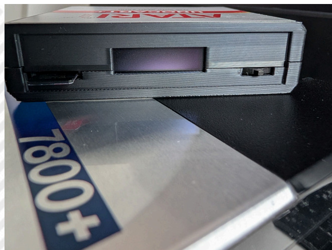
MicroSD slot, OLED display and navigation selector
