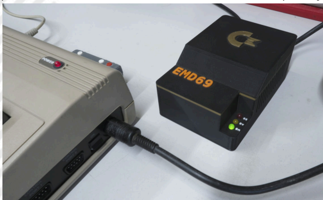
The ALMC64U power supply at work
