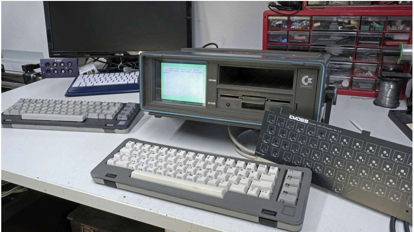
KBSX64U keyboard and membrane in operation on an SX-64
